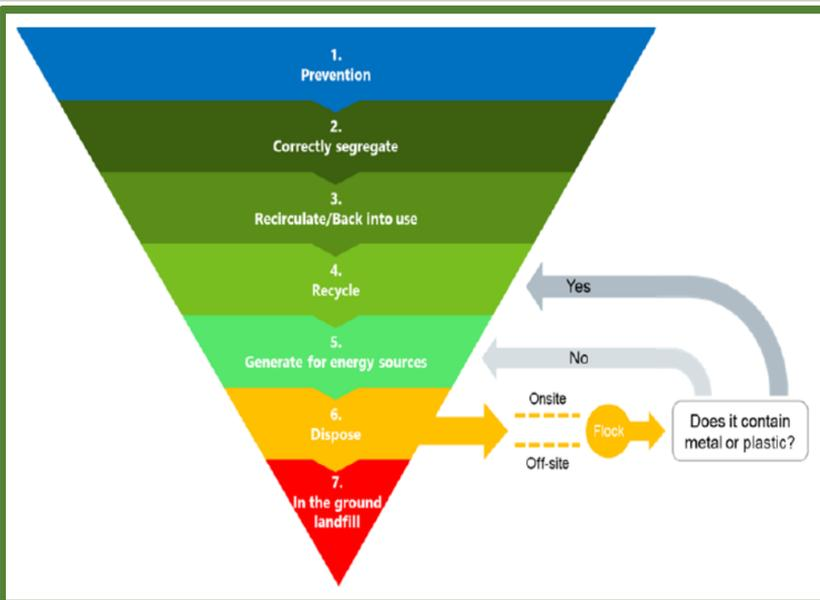
The Waste Hierarchy (adapted for clinical waste) is left. It is self-explanatory with the aim of encouraging most effort on waste prevention with the aim of reducing waste arising at each subsequent level of the Hierarchy.
